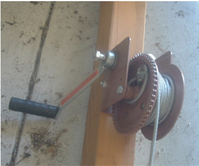
The winch attached with 3 bolts through the 4X4.
