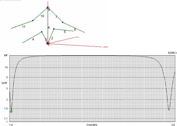
Still much past work with EZNEC results being translated into real antennas has taught that the model is just a general guide (especially for wires near the ground) yet it is very useful when predicting the changes in impedance from small changes in lengths. Pruning, aided by the ever popular MJF, will be necessary and nothing is guaranteed.
