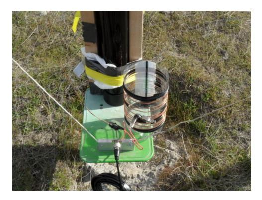
Note that the "beverage" coil form could also serve as a rain gauge unless drain holes are used. The less that elegant temporary 2 element choke is shown below.
