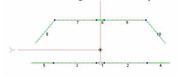
First the driven element alone was evaluated for length required for a 24.9 MHz resonance. Using that drive length, the reflector was added with the wire sections (8 and 10) adjusted in length to get a useful radiation pattern with yagi-like gain. As the length is varied, the antenna pattern changes with passive element being a director or reflector or a bidirectional pattern between. A reflector length was found by trial and error with EZNEC. But you are not done.
