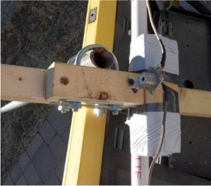
Mast attachment, feed point and DE support (yellow part is a saw horse).
